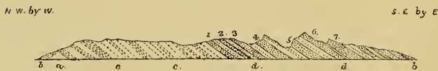
Fig. 6.—Section across the Alicoor hills, from north-west by west to south-east by east. a, Gneiss; c, Sripermatoor group; d, Sattavedu group; e, talus. Nos. 1—7. Conglomerate beds.
