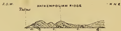
Fig. 5.—Ideal section from Chinnareddypolliam to Hodson's Pettah hill. a, Gneiss; b, Runs of quartzite bed; c, Sripermatoor group; d, Sattavedu group.
